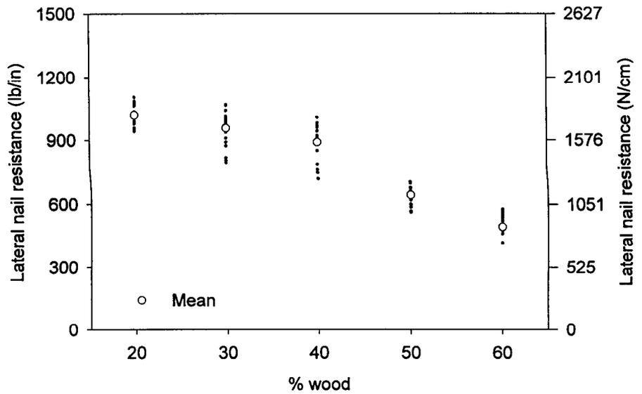
Figure 5. – Lateral nail resistance test results.
