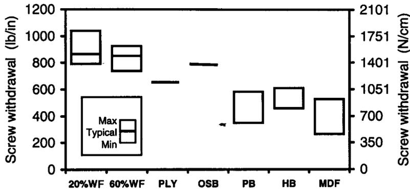
Figure 8. – Comparison of screw withdrawal resistance for wood-plastic composites and conventional wood panel products; WF = wood flour content by weight; PLY = plywood; OSB = oriented strandboard; PB = particleboard; HB = hardboard; MDF = medium density fiberboard.
