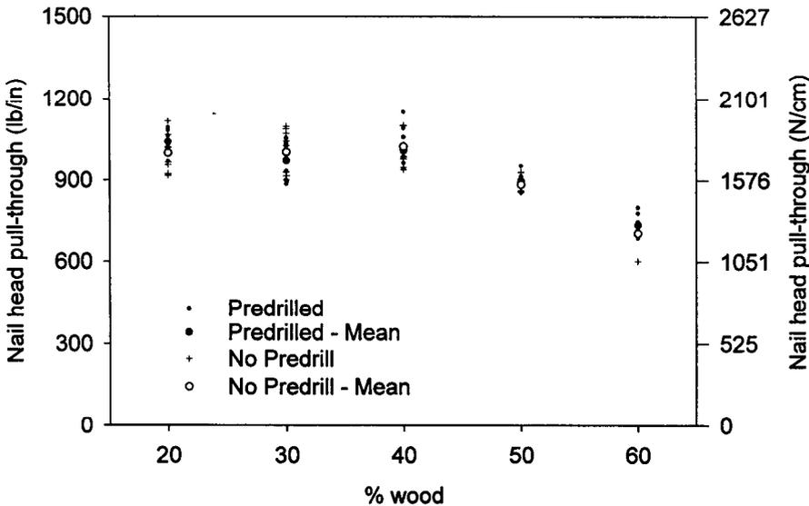
Figure 7. – Effect of predrilling on nail head pull-through.
