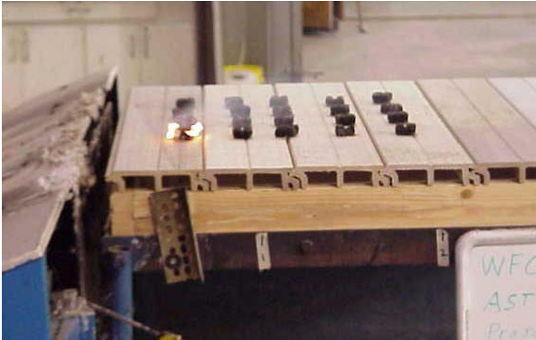
Figure 3. WPC 2 fire propagation test after 20 minutes.
