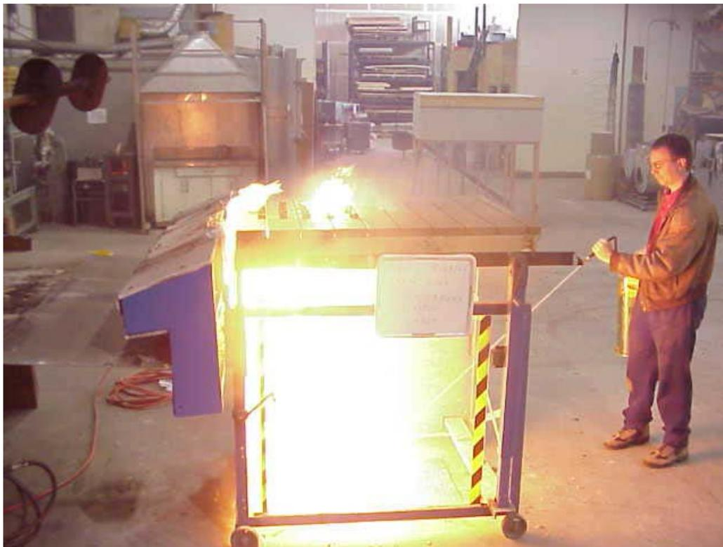
Figure 4. Plastic lumber fire propagation test after 29 minutes.
